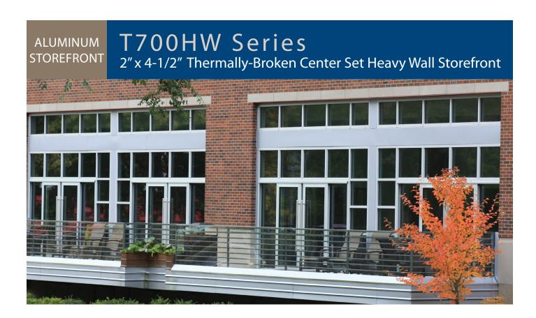
The D8 Aluminum T700HW Series Storefront is a thermally-broken screw spline center set heavy wall storefront system that delivers high-energy efficiency and is a cost-effective glazing solution for commercial construction. This Series can accommodate all standard PAC entrances and vents. It comes in a wide variety of custom painted and anodized finishes.
